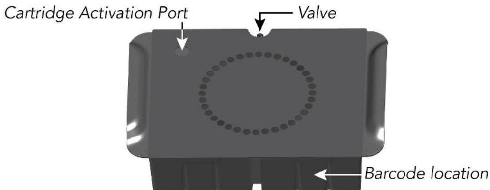
7. With a 1-mL pipette set to 1 mL, carefully add all the Imaging Activation Mix via the Cartridge Activation Port by inserting the pipette tip below the level of the liquid in the MERSCOPE Imaging Cartridge before dispensing. **Without changing** the pipette tip, lower and raise the pipette plunger **10x** at moderate speed to thoroughly mix the solution in the imaging cartridge, but without introducing air bubbles.
