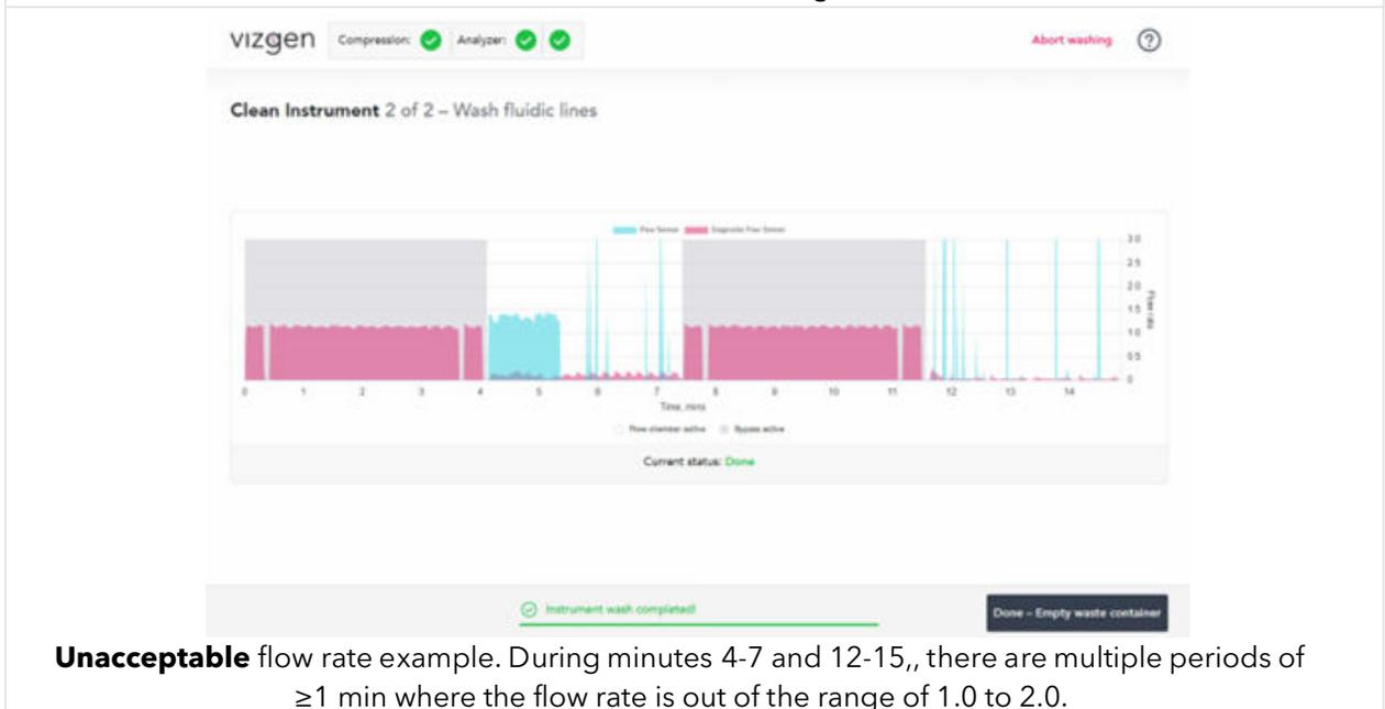
**Unacceptable** flow rate example. During minutes 4-7 and 12-15,, there are multiple periods of  $\geq 1$  min where the flow rate is out of the range of 1.0 to 2.0.
