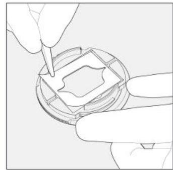
Place the gasket on top of the MERSCOPE slide. Ensure orientation is correct.
