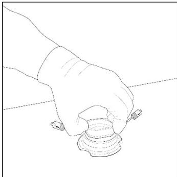
Insert the aqueduct. Ensure the notch in the base and flow direction arrows are oriented correctly.
