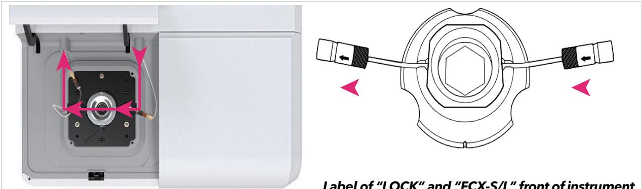
The MERSCOPE Instrument pulls fluid from right to left (pink arrows indicate the direction of flow).
