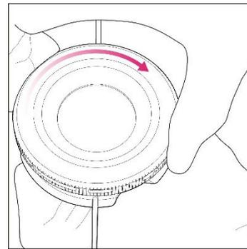
Align and twist the top clockwise until the **Lock** markings on the top and base are aligned.
