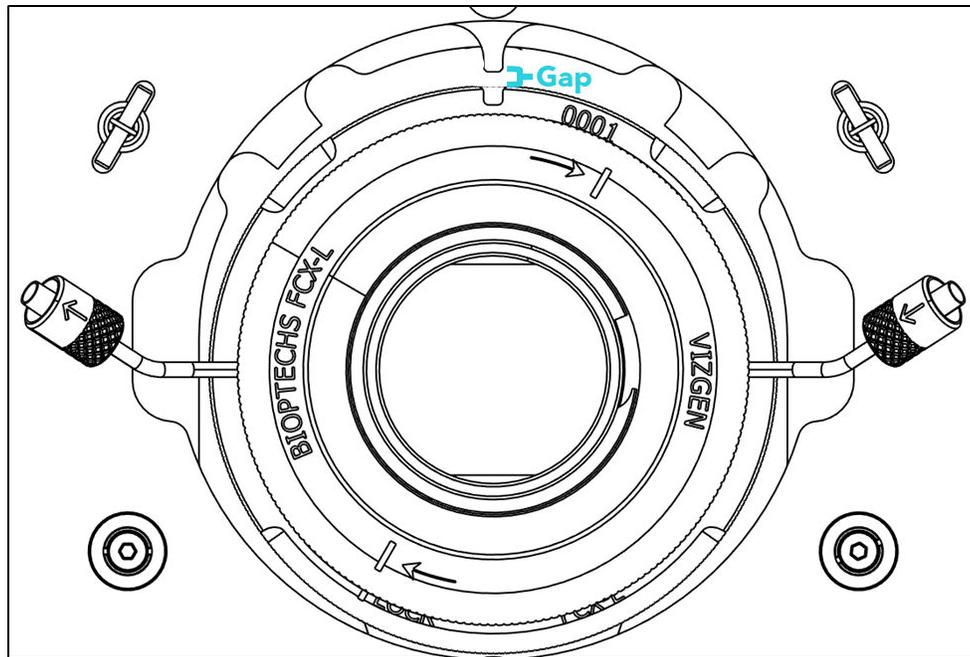
16. Once the flow chamber is lying flat on the stage adapter, gently push the flow chamber toward the 12 o'clock position so the notch is engaged with the tab on the stage adapter. Note: By design, the tab will not sit flush against in the notch. Below image and the inset shows proper positioning and approximate gap size, respectively. If there is no gap, or if the gap is excessive, the flow chamber has not been installed correctly.
