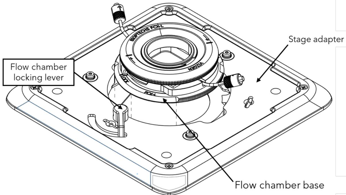
14. Start by locating the notch on the top plate of the flow chamber base (circled below) and orient the flow chamber so the notch is at the 12 o'clock position. Also, confirm the flow chamber locking lever on the stage adapter is in the open (counterclockwise) position.
