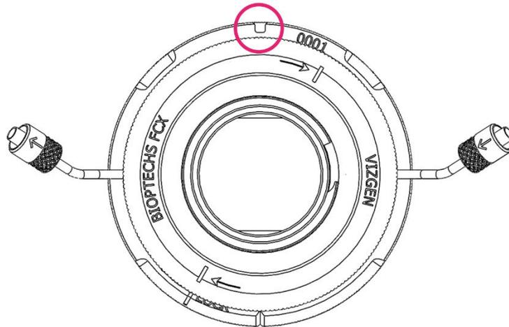
15. Lower the flow chamber into the stage adapter by first inserting the back of the flow chamber under the overhangs at 10 and 2 o'clock then rest the front of the flow chamber flat on the stage adapter. Looking down at the flow cell, it should be approximately positioned as shown below.
