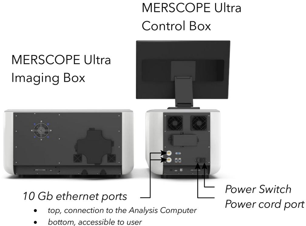
The MERSCOPE Ultra Instrument is a combination of the MERSCOPE Ultra Imaging Box and MERSCOPE Ultra Control Box, where the instrument is programmed via an intuitive touchscreen user interface. The MERSCOPE Ultra Analysis Computer processes the images acquired on the instrument to generate the list of detected transcripts, mosaic images, and cell segmentation results.
