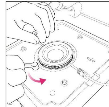
Remove the flow chamber from the stage adapter and disassemble
