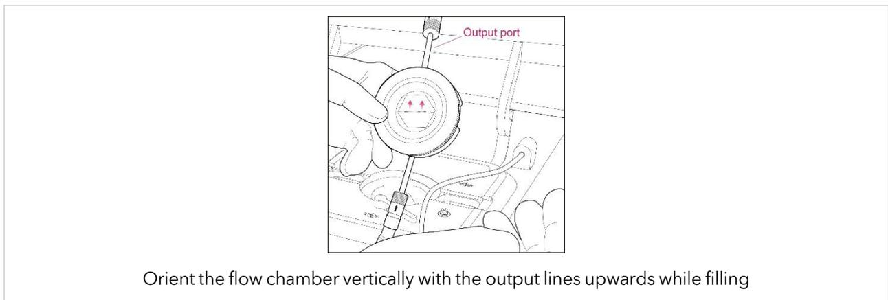
Orient the flow chamber vertically with the output lines upwards while filling
