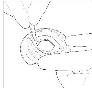
Place the gasket on top of the MERSCOPE slide. Ensure orientation is correct.
