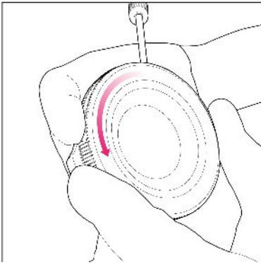
Rotate the Top counterclockwise to disassemble the flow chamber. Clean the gasket, base, and aqueduct
