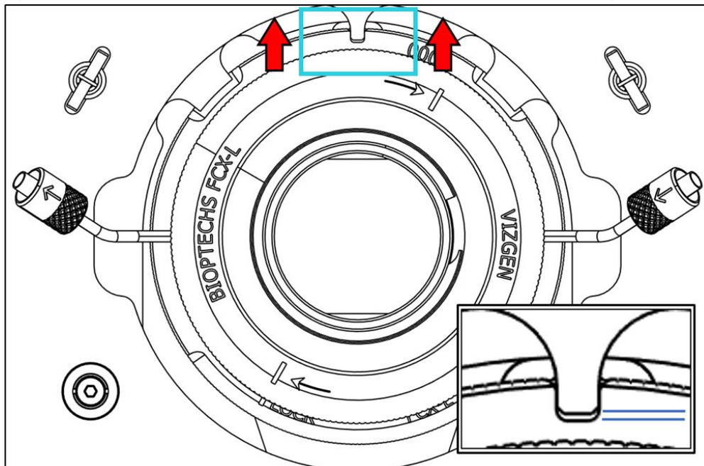
17. Lock the flow chamber into place by rotating the locking lever clockwise. The lever should be tightened by hand until firm resistance is felt. The lever may not travel to the end of the groove. Overtightening may cause damage to the locking mechanism. When tightened appropriately, the flow chamber will be secure, and the brass locking mechanism will be visible against the 6 o'clock position of the flow chamber base (circled below).
