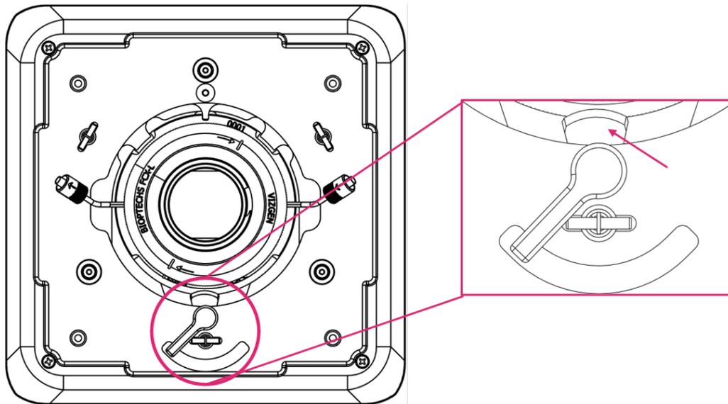
18. Feed any excess inlet and outlet tubing back into the instrument to avoid the tubing from getting caught when closing lid.
