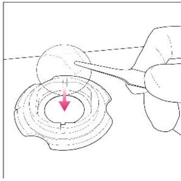
Place the new MERSCOPE Slide in the base with sample gel facing up
