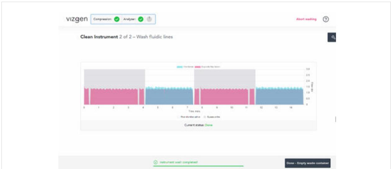
**Acceptable** flow rate example. During minutes 4-7 and 12-15, there are no periods of  $\geq 1$  min where the flow rate is out of the range of 1.0 to 2.0.
