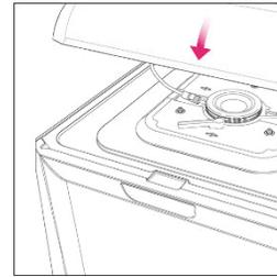
Return the flow chamber to the stage adapter. Close the flow chamber lid
