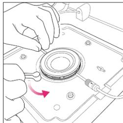
Unlock the flow chamber. Remove the flow chamber from the stage adapter but **DO NOT DETACH** the fluidic lines
