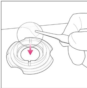
Place the new MERSCOPE Slide in the Base, sample gel facing up
