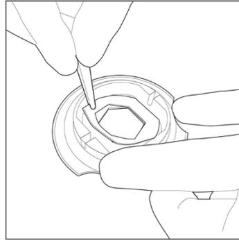
Place the MERSCOPE Gasket on top of the MERSCOPE Slide. Refer to previous page for correct gasket orientation
