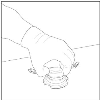
Assemble the Aqueduct. Ensure the notch in the Base and the flow direction arrows marked on the Aqueduct connectors are oriented correctly
