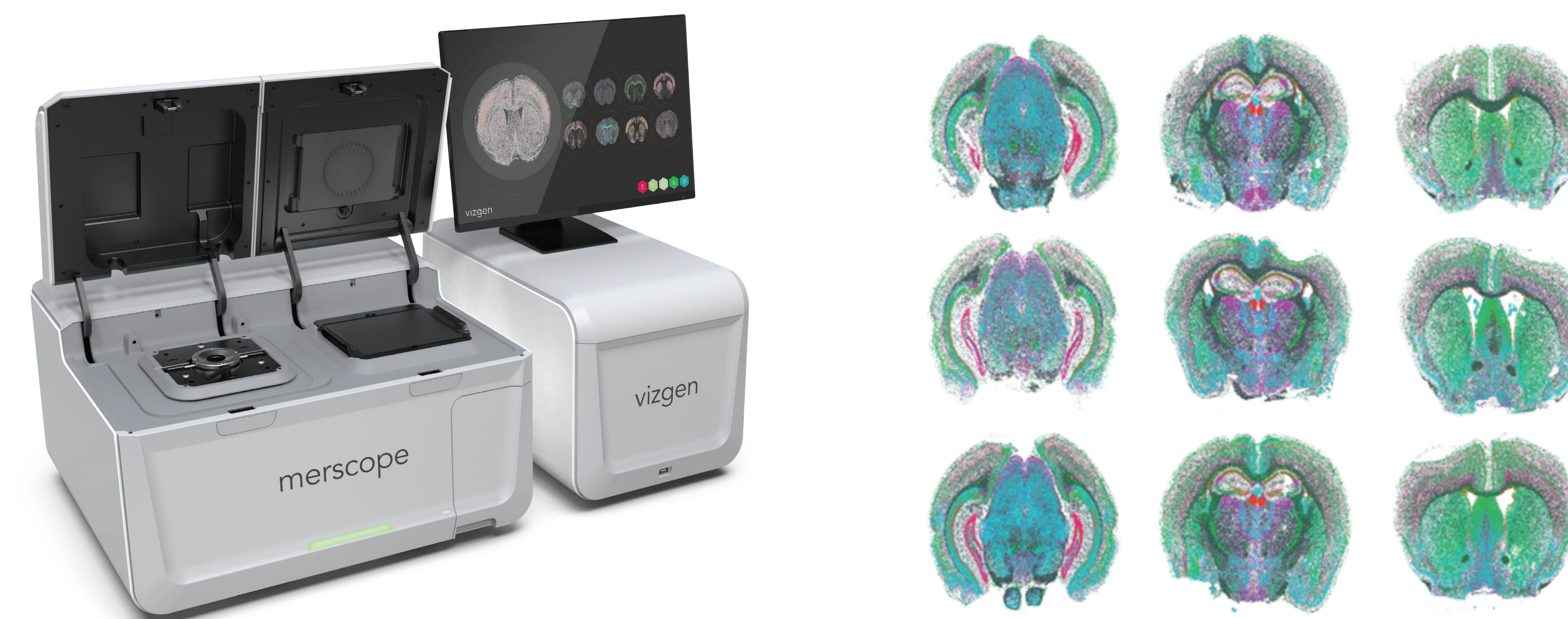
FIGURE 3. Vizgen MERSCOPE Platform. The MERSCOPE platform contains a high resolution fluorescence imaging system to perform the single molecule imaging required for MERFISH and a fluidic system for extinguishing the signal and retaining between each imaging round to automatically perform a full MERFISH measurement.
